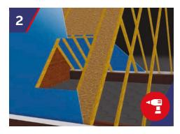
Fix 18mm plywood support between rafters. Ensuring the plywood is the same height as the top of the truss line. Fix roofing felt to roof. Only the area under the dormer needs to be felted during the lifting and fitting of the dormer.
