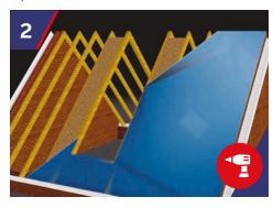
Fix 18mm plywood support between rafters. Ensuring the plywood is the same height as the top of the truss line. Fix roofing felt to roof. Only the area under the dormer needs to be felted during the lifting and fitting of the dormer.
