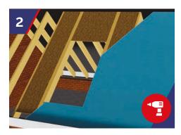
Fix 18mm plywood support between rafters. Ensuring the plywood is the same height as the top of the truss line.
