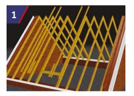
Rafters to be set out to meet side cheek framing. Trimming Rafters to be positioned under side cheeks with outer edge of outer most trimmer in line with GRP side cheek. Trimmers to be positioned 18mm below to the top of the trusses.
