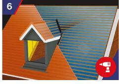
Batten out roof for tiling. Ensure the timber cocking fillet is installed creating a constant fall from the dormer onto the first row of tiles below the dormer. Using full and half tiles (tile and half preferred) set tiles within a maximum of 15mm from the side of the GRP dormer roof. This inside tile now covers the foam strip. Drill and nail all abutment tiles and adjacent tiles.
