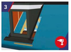
Fix timber cocking fillet to support lead. Lift GRP Dormer into place onto roof. Timber fillet can be positioned at a later date if the roof isn't being finished at the same time as the dormer installation.
