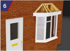
The roof will need to be insulated with suitable depth of quilt insulation prior to tiling the roof. Roofs can then be traditionally tiled and lead flashed to manufacturer's instructions.
