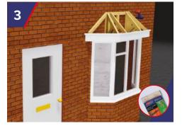
Insert StormFix Blue Fixing sleeve 120 into the drilled holes.
