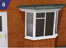
The bay window roof must be over flashed with lead flashing to the Lead Associations recommendations and on exposed sites a bead of sealant/lead adhesive is applied to avoid lifting the flashing.
