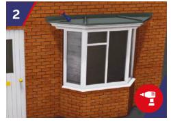
Using a 10mm drill bit, drill through the GRP Upstand into wall structure at a maximum of 450mm centres, to suit the StormFix 80 Fixing.
