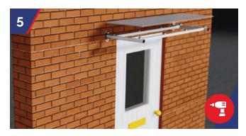
Place the polycarbonate sheet onto the glass spacers with the pole studs passing through the pre-drilled holes in the sheet. Remove the film from the underside of the polycarbonate sheet.
