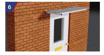
Place remaining threaded glass clamps and rubber washer seals on top of polycarbonate sheet. Remove the film from the top of the polycarbonate sheet. Working from the centre outwards loosely tighten the glass clamps onto the pole studs. Fully tighten the pole fixings and then all the glass clamps.
