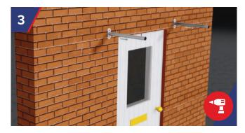
Loosely secure poles to wall in pre-drilled holes, with StormFix 80 Fixing provided. Place plastic end caps to support poles. Lay cross bars onto support poles with vertical section of bar facing front.
