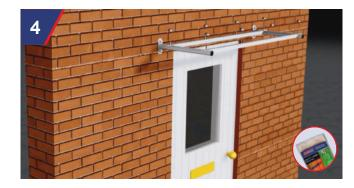
Place the plain bottom glass spacers and rubber washer seals onto each of the pole studs.
