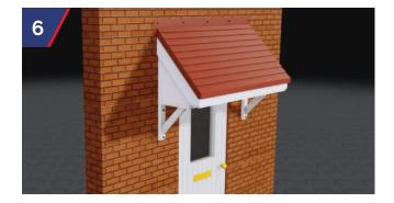
The Gallows Brackets are fixed to the canopy soffit in two places on each bracket. The Gallows Brackets are NOT to be used as the main structural support for the canopy. The upstand must be over flashed in lead or mastic sealed.
