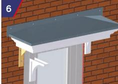
GRP Kneeler to cloak the timber insert and to be either bonded into position or screw fixed from the side into the timber insert. Canopy GRP upstand must be over flashed in lead or mastic sealed back to the structure.
