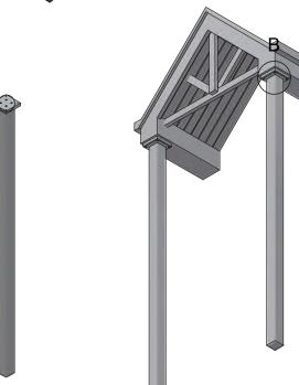
Secondly attach the post plate to the underside of the canopy through the outer post plate holes using 5mm x 50mm (min length) wood screws.
