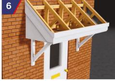
The Gallows Brackets are fixed to the canopy soffit in two places on each bracket. The Gallows Brackets are NOT to be used as the main structural support for the canopy. All tiling battens should be secured to all support trusses. The roofs can be traditionally tiled to tile manufacturer's recommendations.
