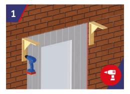
GRP Kneeler supplied with a timber insert. Position Timber Inserts ensuring correct position in relation to the canopy and they are level. Using 10mm drill bit drill through the insert and wall structure to take the StormFix 120 fixing two per insert. Secure the inserts back to the structure. Gallows Brackets are to be fitted following the same method.
