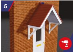
Once the StormFix Blue Fixing Sleeves have been inserted into the holes, fully screw the StormFix 80 fixings into the sleeves.
