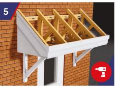
Once the StormFix Blue Fixing Sleeves have been inserted into the holes, fully screw the StormFix 120 fixings into the sleeves.
