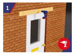
Position template central to the opening and the desired height. Using the centre of the 3 holes drill hole for fixing. Fix one side of template to wall, level up and repeat for other side of template.
