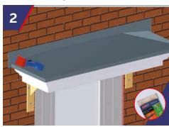
The canopy is placed onto the bracket inserts. Using 10mm drill bit, drill through the GRP upstand and into the wall structure at a maximum of 450mm centres, to suit StormFix 80 fixings.
