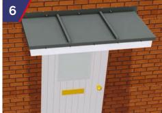
GRP Roof downstand to be fixed to GRP base using fir tree fixings as supplied. The upstand must be over flashed in lead or mastic sealed.
