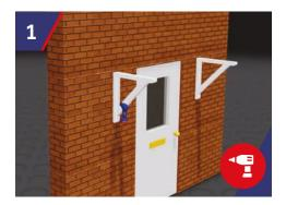
The Gallows Brackets are fixed into the wall in two places ensuring the gallows are level. Using a 10mm drill bit, drill into wall structure, to suit the StormFix 120 Fixing. Insert StormFixBlue Frame Fixing Sleeve 120 into the drilled holes.
