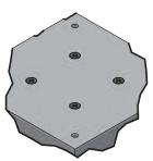
Firstly attach the post plate to the top of the post through the central post plate holes using 5mm x 50mm (min length) wood screws.
