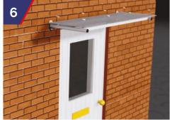
Place remaining threaded glass clamps and rubber washer seals on top of polycarbonate sheet. Remove the film from the top of the polycarbonate sheet. Working from the centre outwards loosely tighten the glass clamps onto the pole studs. Fully tighten the pole fixings and then all the glass clamps.
