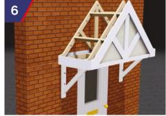
The Gallows Brackets are fixed to the canopy soffit in two places on each bracket. The Gallows Brackets are NOT to be used as the main structural support for the canopy. All tiling battens should be secured to all support trusses including the back truss against the structure. The roofs can be traditionally tiled to tile manufacturer's recommendations.
