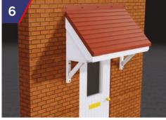
The Gallows Brackets are fixed to the canopy soffit in two places on each bracket. The Gallows Brackets are NOT to be used as the main structural support for the canopy. The upstand must be over flashed in lead or mastic sealed.
