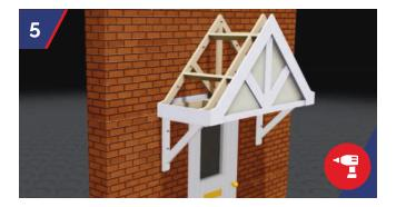
Once the StormFix Blue Fixing Sleeves have been inserted into the holes, fully screw the StormFix 120 fixings into the sleeves.
