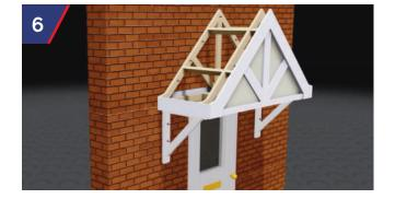
The Gallows Brackets are fixed to the canopy soffit in two places on each bracket. The Gallows Brackets are NOT to be used as the main structural support for the canopy. All tiling batterns should be secured to all support trusses including the back truss against the structure. The roofs can be traditionally tiled to manufacturer's recommendations.
