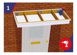
With canopy base in the desired position use a 10mm drill bit, drill through the rear structural timber rail into wall structure at a maximum of 450mm centres, to suit the StormFix 120 Fixing. The centre hole of the MS steel brackets can be used if appropriate.
