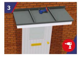
The roof unit is positioned onto the base unit. Using a 10mm drill bit, drill through the GRP upstand into wall structure at a maximum of 450mm centres, to suit the StormFix 80 Fixing.
