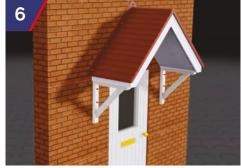
The Gallows Brackets are fixed to the canopy soffitt in two places on each bracket. The Gallows Brackets are NOT to be used as the main structural support for the canopy. The upstand must be over flashed in lead or mastic sealed.
