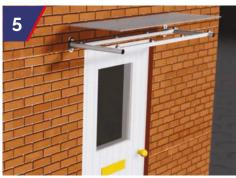
Place the polycarbonate sheet onto the glass spacers with the pole studs passing through the pre-drilled holes in the sheet. Remove the film from the underside of the polycarbonate sheet.
