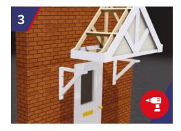
The canopy is placed on the brackets. Using a 10mm drill bit, drill through the rear structural timber truss into wall structure at a maximum of 450mm centres, to suit the StormFix 120 Fixing.
