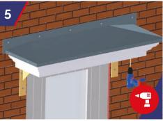
Kneeler Brackets inserts are fixed to the canopy soffit in twoplaces on each bracket using wood screws (not supplied). Gallows Brackets to be secured to the soffit following the same method. Please note the Gallows / Kneelers are only supporting the soffit of the canopy and shouldn't be used as the main support
