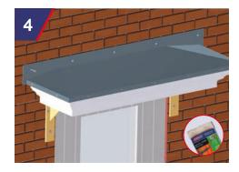
Once the StormFix fixing sleeves have been fully inserted into the holes, fully screw the StormFix 80 screw into the sleeves. Screws & sleeves to be concealed using the caps supplied loose with the fixings.
