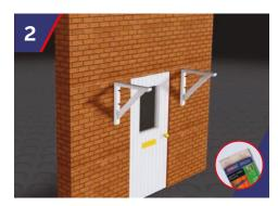
Once the StormFix Blue Frame Fixing Sleeves have been inserted into the holes, fully screw the StormFix 120 fixings into the sleeves.
