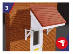
The canopy is placed on the brackets. Using a 10mm drill bit, drill through the GRP Upstand into wall structure at a maximum of 450mm centres, to suit the StormFix 80 Fixing.
