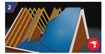
Fix 18mm plywood support between rafters. Ensuring the plywood is the same height as the top of the truss line. Fix roofing felt to roof. Only the area under the dormer needs to be felted during the lifting and fitting of the dormer.
