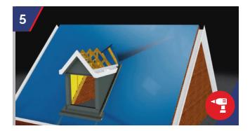
100mm x 75mm framing clamps screw fixed to side cheek framing and nailed or screw fixed to support rafters. Supplied and fitted by others, on site. Minimum of 3 No. per dormer side.
