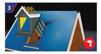
Fix timber cocking fillet to support lead. Lift GRP Dormer into place onto roof. Timber fillet can be positioned at a later date if the roof isn't being finished at the same time as the dormer installation.
