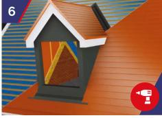
Batten out roof for tiling. Ensure the timber cocking fillet is installed creating a constant fall from the dormer onto the first row of tiles below the dormer. Using full and half tiles (tile and half preferred) set tiles within a maximum of 15mm from the side of the GRP dormer roof. This inside tile now covers the foam strip. Drill and nail all abutment tiles and adjacent tiles.
