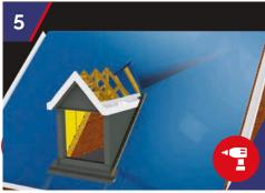
100mm x 75mm framing clamps fixed to side cheek framing, nailed or screw fixed to support rafters. Supplied and fitted by others, on site. Minimum of 3 No. per dormer side.
