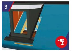
Fix timber cocking fillet to support lead. Lift GRP Dormer into place onto roof. Timber fillet can be positioned at a later date if the roof isn't being finished at the same time as the dormer installation.
