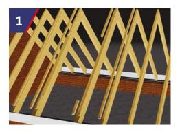
Rafters to be set out to meet side cheek framing. Trimming rafters to be positioned under side cheeks with outer edge of outer most trimmer in line with GRP side cheek. Trimmers to be positioned 18mm below to the top of the trusses.
