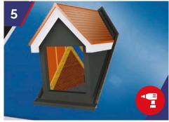
100mm x 75mm framing clamps fixed to side cheek framing, nailed or screw fixed to support rafters. Supplied and fitted by others, on site. Minimum of 3 No. per dormer side.
