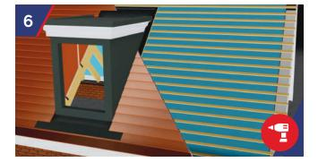
Battern out roof for tiling. Ensure the timber cocking fillet is installed creating a constant fall from the dormer onto the first row of tiles below the dormer. Using full and half tiles (tile and half preferred) set tiles within a maximum of 15mm from the side of the GRP dormer roof. This inside tile now covers the foam strip. Drill and nail all abutment tiles and adjacent tiles.
