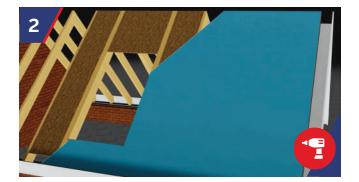
Fix 18mm plywood support between rafters. Ensuring the plywood is the same height as the top of the truss line. Fix roofing felt to roof. Only the area under the dormer needs to be felted during the lifting and fitting of the dormer.
