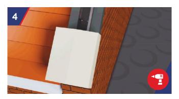
For fitting COPEKING® stop end, take length of strap within clip pack supplied with each stop end. Attach half of strap to underside of stop end using 2 no. screws and washers supplied. Clip fit stop end onto fixing rail and slide to desired position. Ensuring the strap is pulled taught, screw fix remaining half of strap down through fixing rail and into parapet wall using x2 remaining screws and washers.
