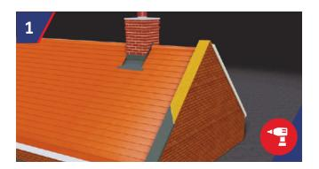
You will require an 18mm exterior quality plywood board to be fixed to the top of the wall. Weather proof the plywood with a polythene DPM or similar and cut off excess to allow 25mm overhang to each side of the plywood.
