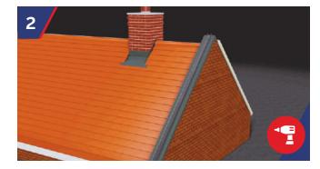
Fix the continous plastic fixing strip to the plywood/DPM using two rows of 5x25mm coated wood screws (not supplied) spaced 60mm apart at 300mm centres. Ensure the fixing strip is central to the wall and adjoining lengths run in line. The fixing strip can be cut to any desired length to suit site conditions.
