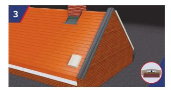
Clip fix all the pre mitred internal, external angles, apex mitres, base mitres and stop end units by firmly pressing COPEKING® down onto the fixing strip until "clicked" into position.
