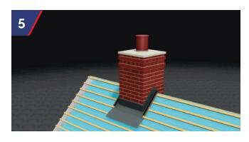
Batten out the roof. Lay a lead support fillet at the base of the chimney to ensure the lead is fully supported and on a continuous downward fall.
