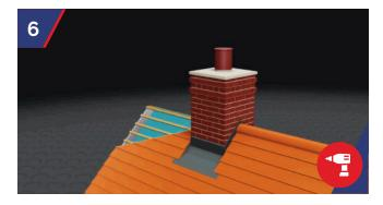
Using full and half tiles (tile and half preferred) set tiles within a maximum of 15mm from the side of the chimney. This inside tile now covers the foam strip. Drill and nail all abutment tiles and adjacent tiles.
