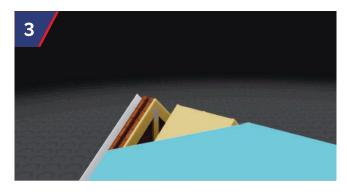
Apply roof felt over all of the roof including over the plywood panels. Only the area under the chimney needs to be felted during the lifting and fitting of the chimney. Lay the SmartStack chimney onto the roofing felt over the plywood panels, using the lifting eye situated within the SmartStack chimney pot.
