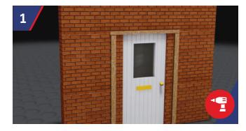
Contractor to fix timber frame securely to wall, by others on site, to suit the size of the GRP door surround.
