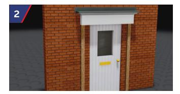
GRP door head to abut wall at base, internal framing will allow canopy to sit over rail with soffit fixing into underside of rail.
