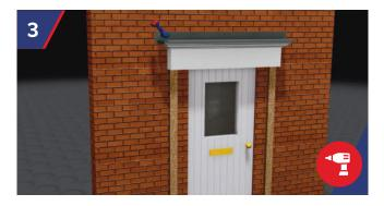
Using a 10mm drill bit, drill through the GRP Upstand into wall structure at a maximum of 450mm centres, to suit the StormFix 80 Fixing.
