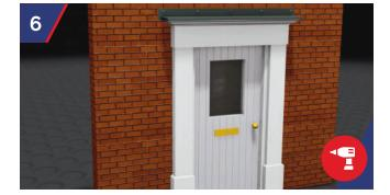
The pilasters are fixed to a timber battern running the full height of the pilaster and fixed into the reveal jamb if applicable. The upstand must be over flashed in lead or mastic sealed.
