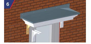
GRP Kneeler to cloak the timber insert and to be either bonded into position or screw fixed from the side into the timber insert. Canopy GRP upstand must be over flashed in lead or mastic sealed back to the structure.
