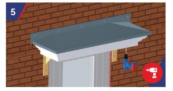
Kneeler Brackets inserts are fixed to the canopy soffit in two places on each bracket using wood screws (not supplied). Gallows Brackets to be secured to the soffit following the same method. Please note the Gallows / Kneelers are only supporting the soffit of the canopy and shouldn't be used as the main support.
