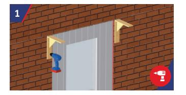
GRP Kneeler supplied with a timber insert. Position Timber Inserts ensuring correct position in relation to the canopy and they are level. Using 10mm drill bit drill through the insert and wall structure to take the StormFix 120 fixing two per insert. Secure the inserts back to the structure. Gallows Brackets are to be fitted following the same method.
