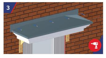
Insert StormFix 80 into the drilled holes. Ensure the canopy is level and maintains a fall to the front.
