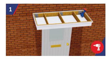
With canopy base in the desired position use a 10mm drill bit, drill through the rear structural timber rail into wall structure at a maximum of 450mm centres, to suit the StormFix 120 Fixing. The centre hole of the MS steel brackets can be used if appropriate.
