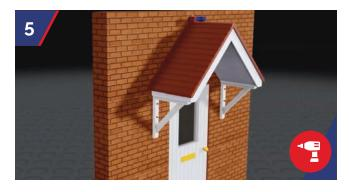
Once the StormFix Blue Fixing Sleeves have been inserted into the holes, fully screw the StormFix 80 fixings into the sleeves.
