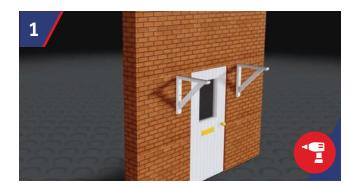
The Gallows Brackets are fixed into the wall in two places ensuring the gallows are level. Using a 10mm drill bit, drill into wall structure, to suit the StormFix 120 Fixing. Insert StormFix Blue Frame Fixing Sleeve 120 into the drilled holes.
