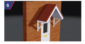
The Gallows Brackets are fixed to the canopy soffitt in two places on each bracket. The Gallows Brackets are NOT to be used as the main structural support for the canopy. The upstand must be over flashed in lead or mastic sealed.
