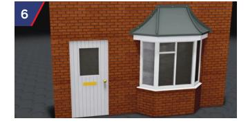
The bay window roof must be over flashed with lead flashing to the Lead Associations recommendations and on exposed sites a bead of sealant/lead adhesive is applied to avoid lifting the flashing.
