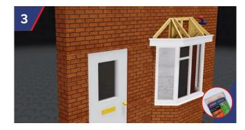
Insert StormFix Blue Fixing sleeve 120 into the drilled holes.
