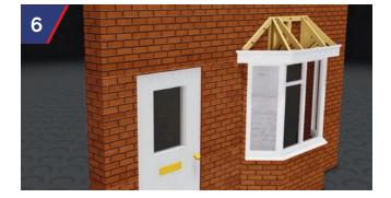
The roof will need to be insulated with suitable depth of quilt insulation prior to tiling the roof. Roofs can then be traditionally tiled and lead flashed to manufacturer's instructions.
