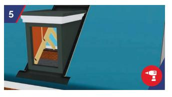
100mm x 75mm framing clamps screw fixed to side cheek framing and nailed or screw fixed to support rafters. Supplied and fitted by others, on site. Minimum of 3 No. per dormer side.
