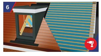
Battern out roof for tiling. Ensure the timber cocking fillet is installed creating a constant fall from the dormer onto the first row of tiles below the dormer. Using full and half tiles (tile and half preferred) set tiles within a maximum of 15mm from the side of the GRP dormer roof. This inside tile now covers the foam strip. Drill and nail all abutment tiles and adjacent tiles.
