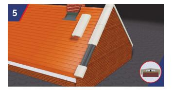
Clip all standard straight lengths between fixed junction units firmly pressing down onto fixing strip until "clicked" into position. If necessary, COPEKING® can be removed by gently prizing one side away from the wall until the holding down clip is released. Repeat for the other side. The white clips factory fitted internally to the COPEKING need to be fully located onto the fixing track as indicated in the above close-up.
