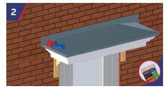
Once the StormFix fixing sleeves have been fully inserted into the holes, fully screw the StormFix 80 screw into the sleeves. Screws & sleeves to be concealed using the caps supplied loose with the fixings.
