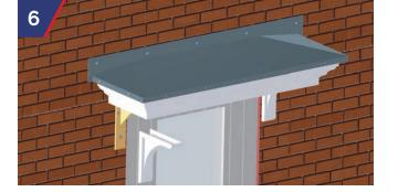
GRP Kneeler to cloak the timber insert and to be either bonded into position or screw fixed from the side into the timber insert. Canopy GRP upstand must be over flashed in lead or mastic sealed back to the structure.
