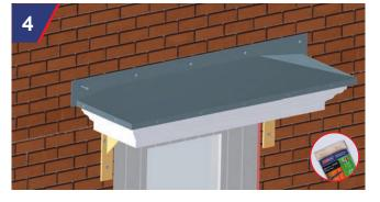
Once the StormFix fixing sleeves have been fully inserted into the holes, fully screw the StormFix 80 screw into the sleeves. Screws & sleeves to be concealed using the caps supplied loose with the fixings.
