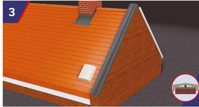
Clip fix all the pre mitred internal, external angles, apex mitres, base mitres and stop end units by firmly pressing COPEKING® down onto the fixing strip until "clicked" into position.
