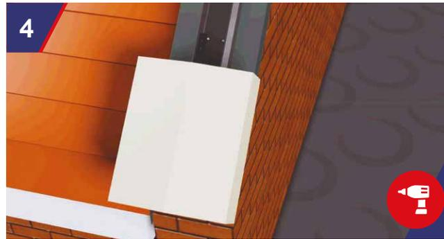
For fitting COPEKING® stop end, take length of strap within clip pack supplied with each stop end. Attach half of strap to underside of stop end using 2 no. screws and washers supplied. Clip fit stop end onto fixing rail and slide to desired position. Ensuring the strap is pulled taut, screw fix remaining half of strap down through fixing rail and into parapet wall using x2 remaining screws and washers.
