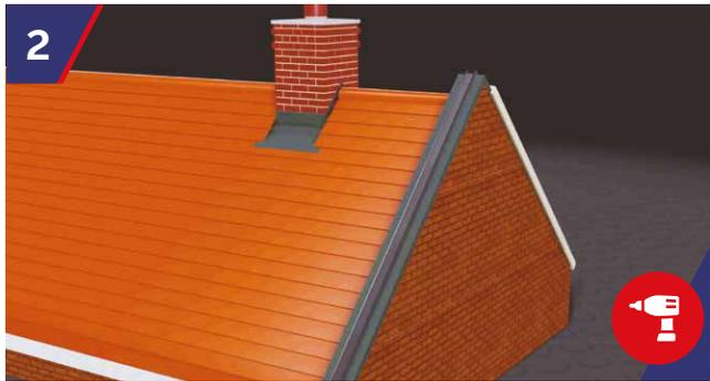
Fix the continuous plastic fixing strip to the plywood/DPM using two rows of 5x25mm coated wood screws (not supplied) spaced 60mm apart at 300mm centres. Ensure the fixing strip is central to the wall and adjoining lengths run in line. The fixing strip can be cut to any desired length to suit site conditions.
