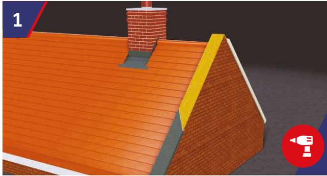
You will require an 18mm exterior quality plywood board to be fixed to the top of the wall. Weather proof the plywood with a polythene DPM or similar and cut off excess to allow 25mm overhang to each side of the plywood.
