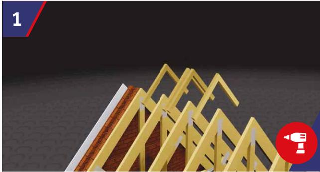
Fix support noggins to the inside of the rafters and insert external quality plywood panels between the rafters ensuring top of plywood is level with top of rafters.
