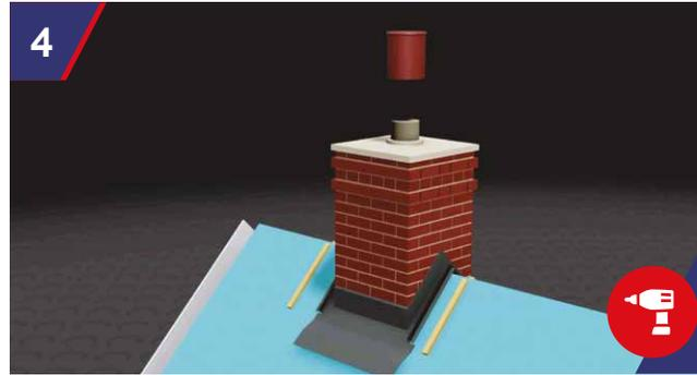
Insert tiling battens under the SmartStack gutter and simultaneously screw fix the GRP gutter and the tiling batten down onto the plywood using the screws supplied through all of the factory drilled holes. Unscrew lifting eye within SmartStack chimney pot and screw on SmartStack chimney pot onto threaded bolt.
