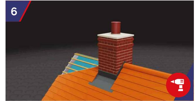
Using full and half tiles (tile and half preferred) set tiles within a maximum of 15mm from the side of the chimney. This inside tile now covers the foam strip. Drill and nail all abutment tiles and adjacent tiles.
