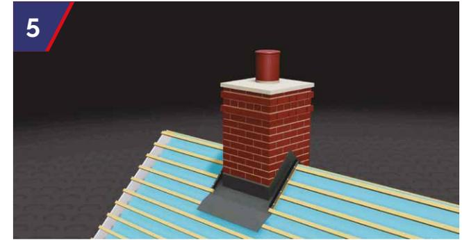
Batten out the roof. Lay a lead support fillet at the base of the chimney to ensure the lead is fully supported and on a continuous downward fall.
