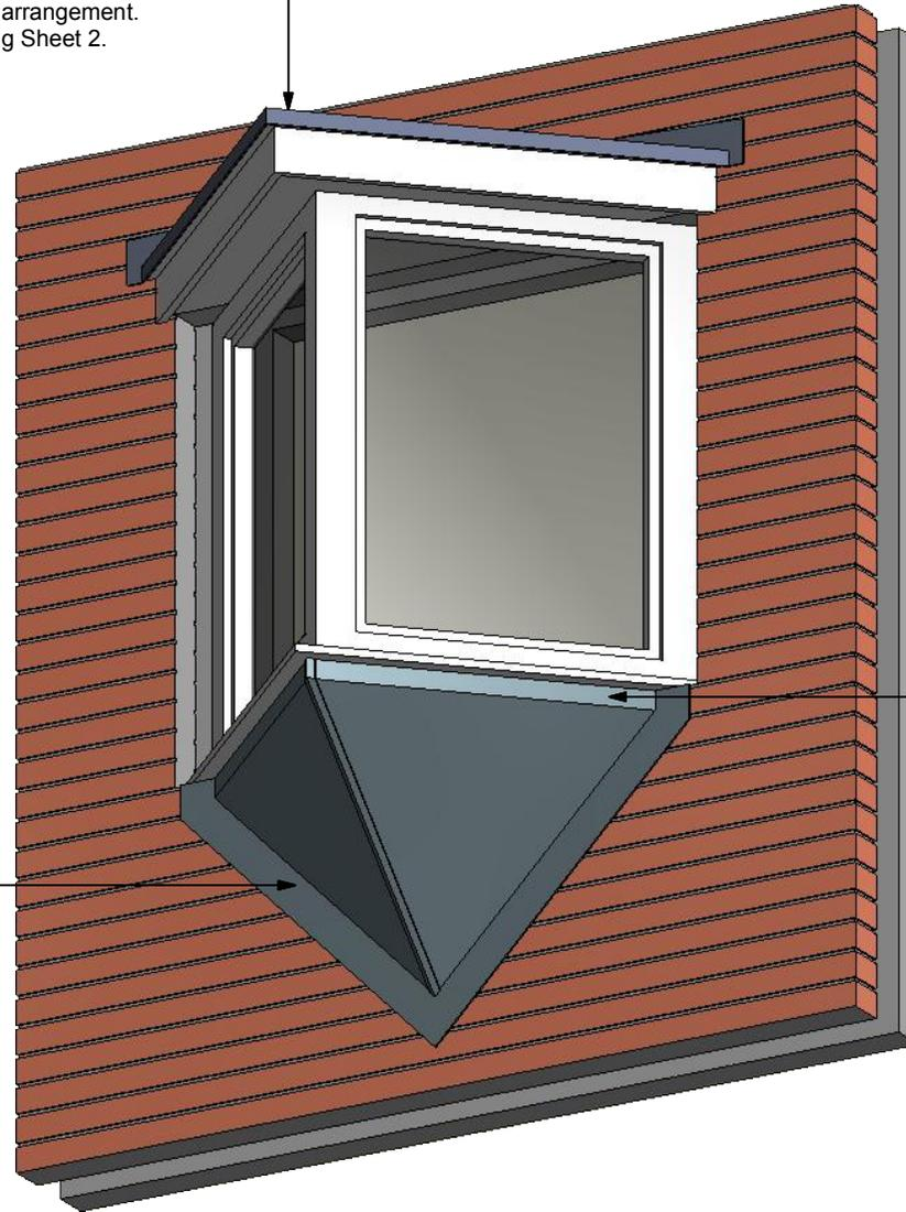
GRP flange to be screw fixed to brickwork at max. 300mm centres all around.
